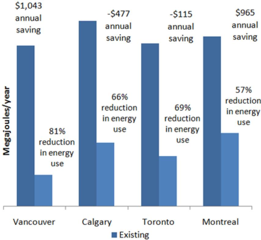
Replacing Gas Furnace (78% eff.) with Air-to-Air Heat Pump
