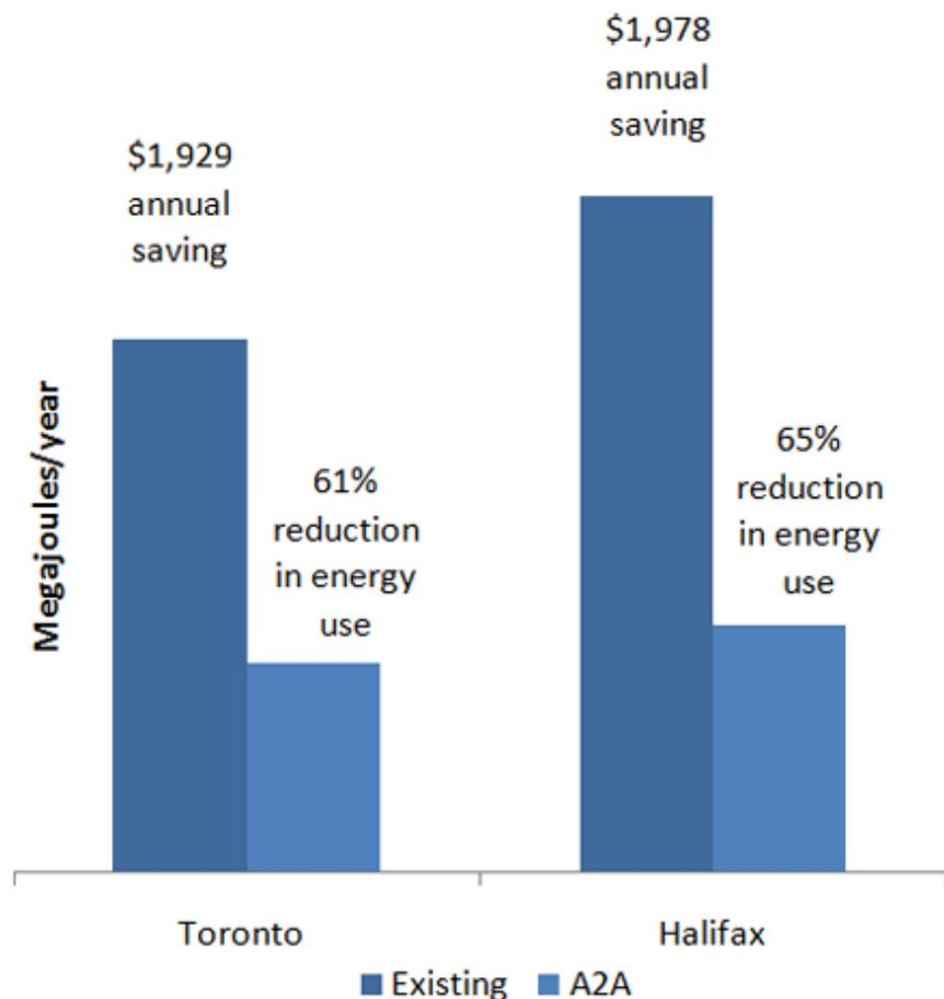
**Replacing Oil Furnace with Heat Pump (A2A)**
